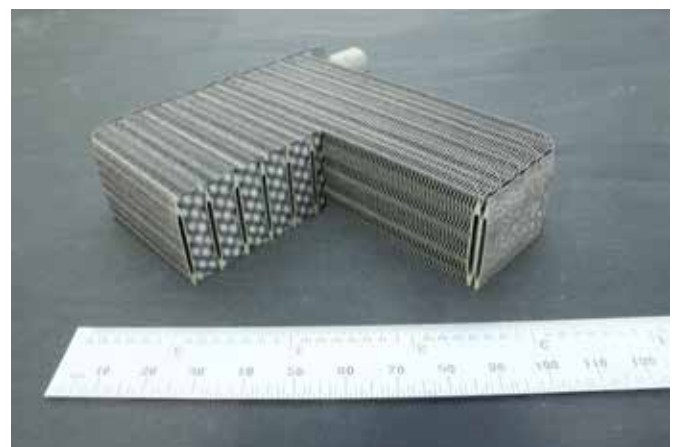
Notional AM part emphasizing ability to fashion unique advanced heat exchanger components with features on the scale of 100 microns. (ARL Released photo)
