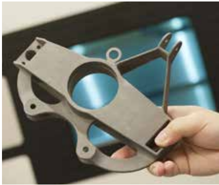
Topological advanced design methodology specimen produced as part of a senior student project demonstrating expanded design space enabled by additive manufacturing. (ARL Released photo)
