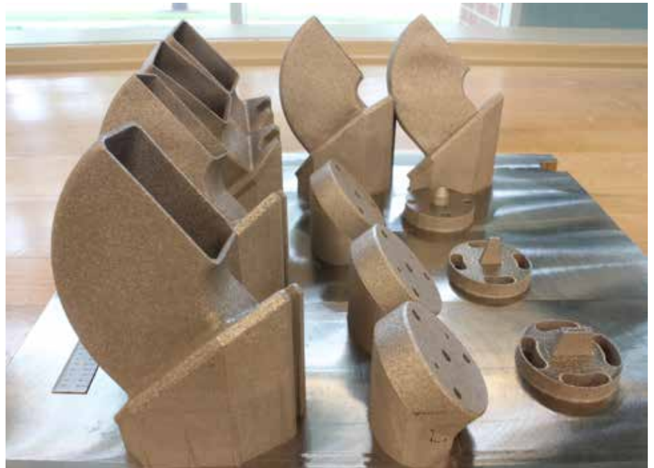
Unmanned Aerial Vehicle (UAV) exhaust components produced through additive manufacturing process. (ARL Released photo)
